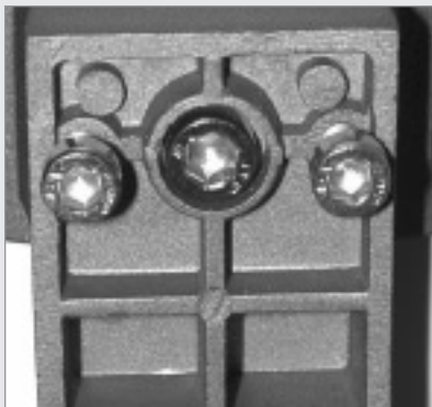
Fig. 47: Cradle adjustment screws.
